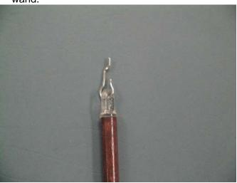
**12.** Push the wand connector clip down and to the side of the tilter stem. Snap wand connector clip down onto the short groove side of the tilter stem.
